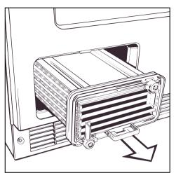
■ Pull out the heat exchanger
